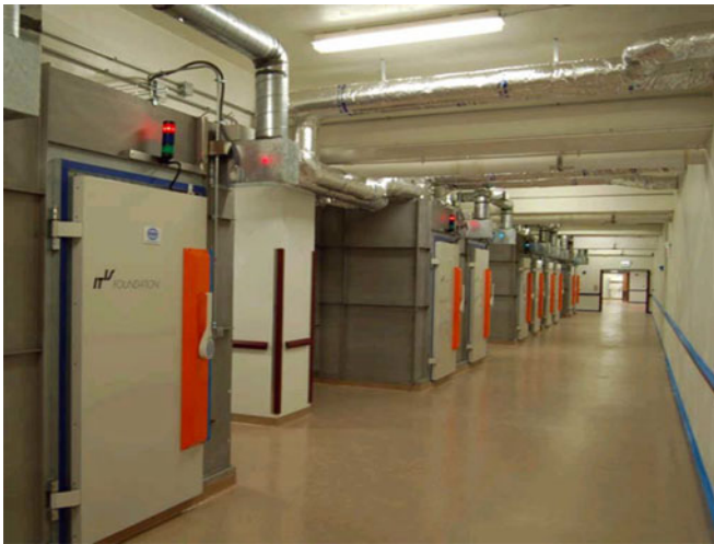
Fig. 5. RFR reverberation chambers installed at IITRI.
